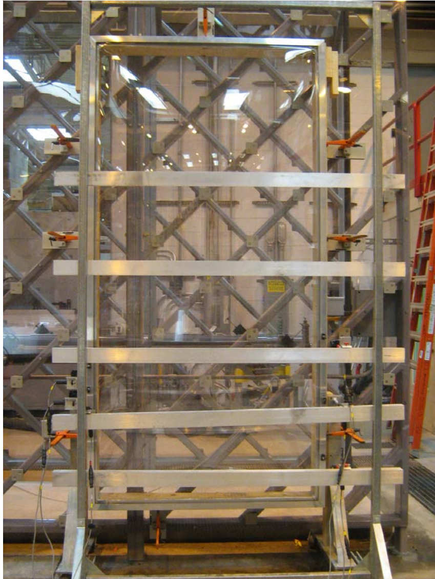
Photo No. 2 Fixed Curb Mount Acrylic Skylight During Structural Testing
